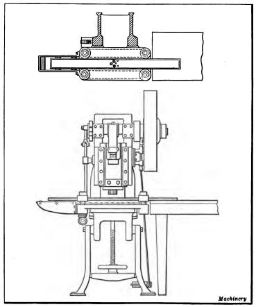
Fig. 5. Press Equipped with Rack-and-pinion Double-roll Feed
